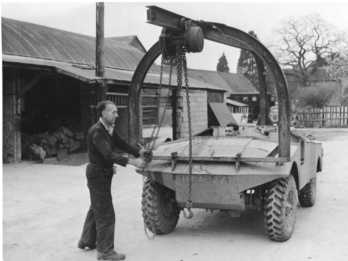
Good use was made of 'war-surplus' equipment on Pit Hall farm, mobile lifting tackle made from a Morris Armoured car, 1948
